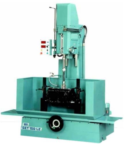
Set 1502 Spindle Rotation Speeds70 o 140rpmSet 150 LEVariable Spindle Rotation Speed40÷150rpm
