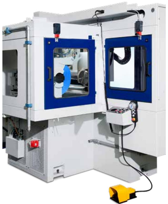
**LATERAL REMOTE HANDWHEEL
